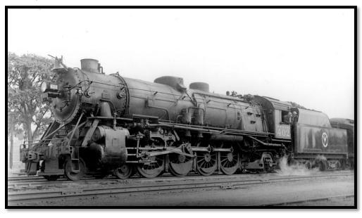
No. 402 here in Passenger train service yet still equipped with the "Booster" engine. Note the footboard pilot, the additional straps from beneath the smokebox in reinforcement of the pilot deck and the steam pipe below the boiler running board in service to the "Booster"
