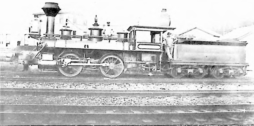
Milt Pulis collection Link and pin coupler is quite visible on the pilot of engine 27. This locomotive was named HUDSON, but by the time of this 1885 photo the practice of naming engines had been dropped.
