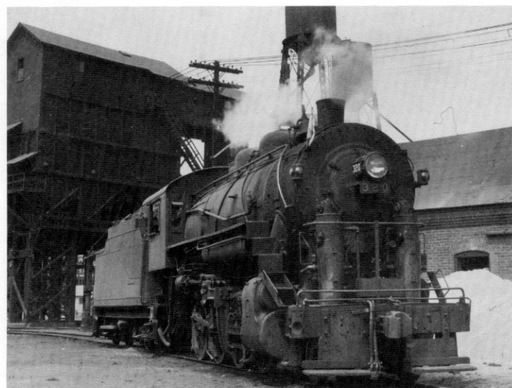
The 320 with pilot mounted air pumps at Middletown. Robert F. Harding photo from Oscar Bennett collection
